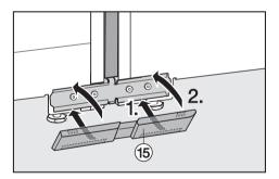
■ Fit cover <sup>(15)</sup> to the bottom of the fronts of the appliances.
